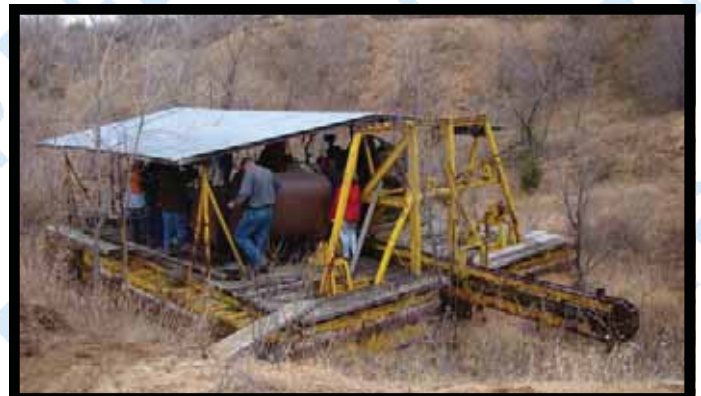
Barge used to mine gravel The high pressure water sprayer at the front of the barge was used to erode the hillside into easily accessible gravel. This barge effectively was used to erode a one-half mile hill.
